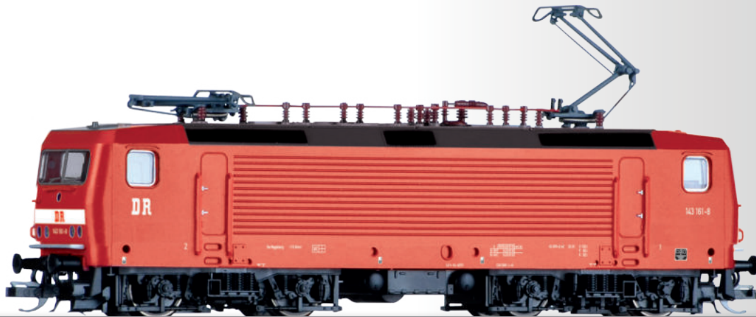
Elektrolokomotive 143 161-8 der DR Electric locomotive 143 161-8 of the DR
